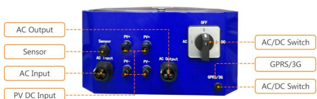
Inverter terminal board
